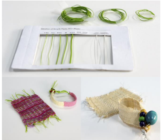
Figure 22: Material from reprocessing the plastic bags to the form of long strings (upper), fabric hand-loomed with the plastic strings as wrap and wool as woof (lower left), and fabric hand-loomed with the plastic strings as wrap, and local natural fibers called raffia as woof. Raffia is made of buri (lower right)
