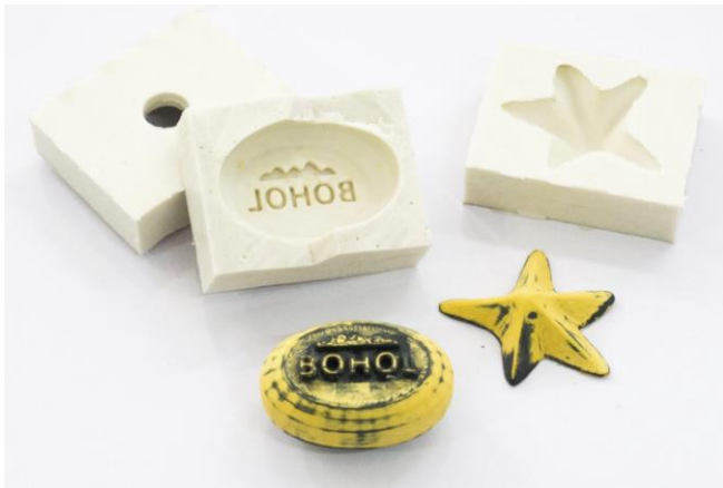
Figure 38: Molds for mass-production produced with a 3D printer provided for a local soap firm
