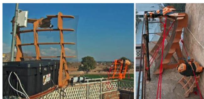
Figure 3: Wooden WiFi router "FabFi" produced at the FabLab in Afghanistan
